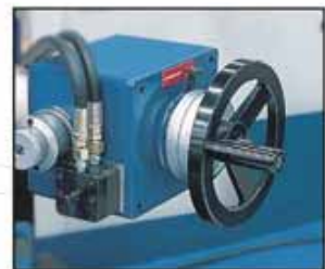
Automatic down feed cycle: plunge-cut and surface grinding modes.
