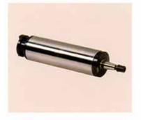
High precision cartridge type wheel spindle with super precision angular contact ball bearings assure accurate grinding performance, bearings are lubricated by grease for life.
