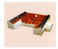
Widely double "V" slideway coated with turcite B and accurately scraped to assure smoothcross feed of the saddle.
