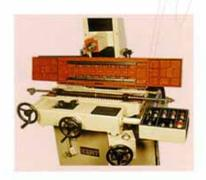
Ball bearing table slideways are used on 250 series for smooth and light movement with extra precision.
